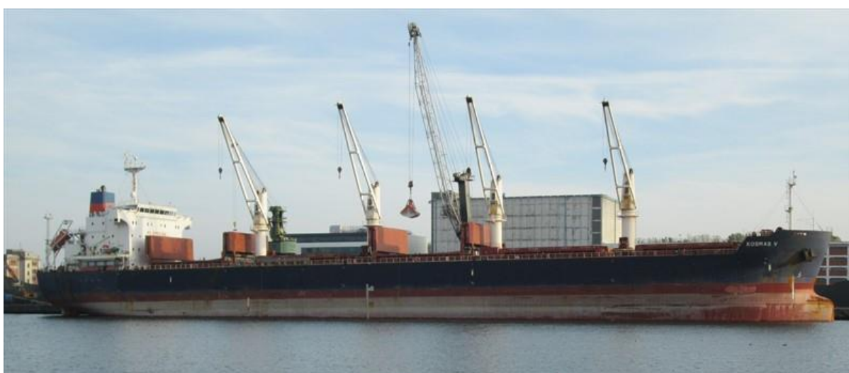
Figure 3.1/1: KOSMAS V cranes and folding type holds' hatch covers.
